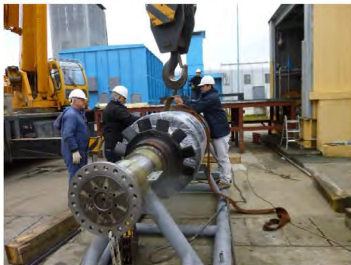
*3.37 APR pumps, SR01 and stop valves TV2C heavy maintenance ,
